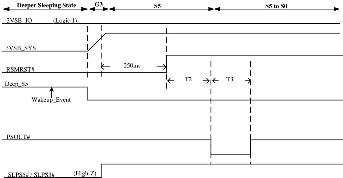
When any Wakeup Event (PSIN#, KB MS Wakeup, CIR wakeup, GPIO Wakeup) happened, pin DEEP\_S5 will be de-asserted to turn on the VSB power to the system. The pin RSMRST# will de-assert when 3VSB\_SYS power reach valid voltage. And then the pin PSOUT# will issue a low pulse (T3) turn on the system after T2 time (wakeup delay time, LD16 CRE0). The PSOUT# low pulse is also programmable (LD16 CRE1). The T4 time is the delay from Deep\_S5 ds-assert to Deeo\_S5#\_DELAY de-assert.
