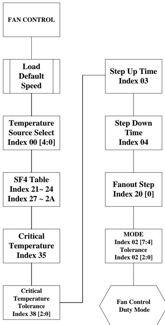
Figure 8-14 Fan Control Duty Mode Programming Flow
