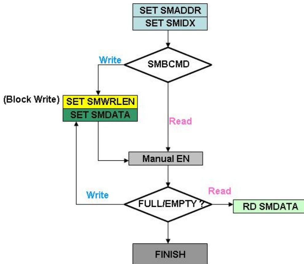
Figure 23-9 Manual Mode Programming Flow
