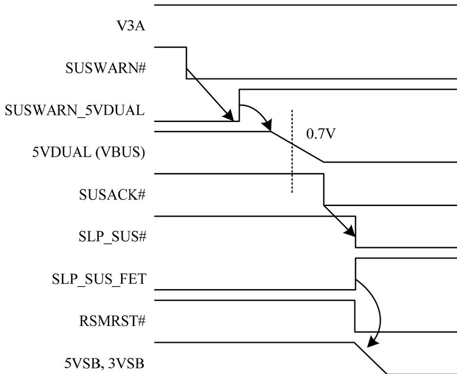
6.9.2 Exit DSW State timing diagram
