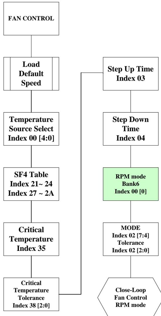
Figure 8-15 Close-Loop Fan Control RPM mode Programming Flow
