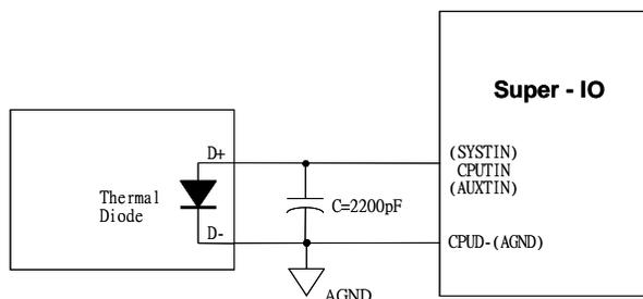
Figure 8-7 Monitoring Temperature from Thermal Diode (Current Mode)
