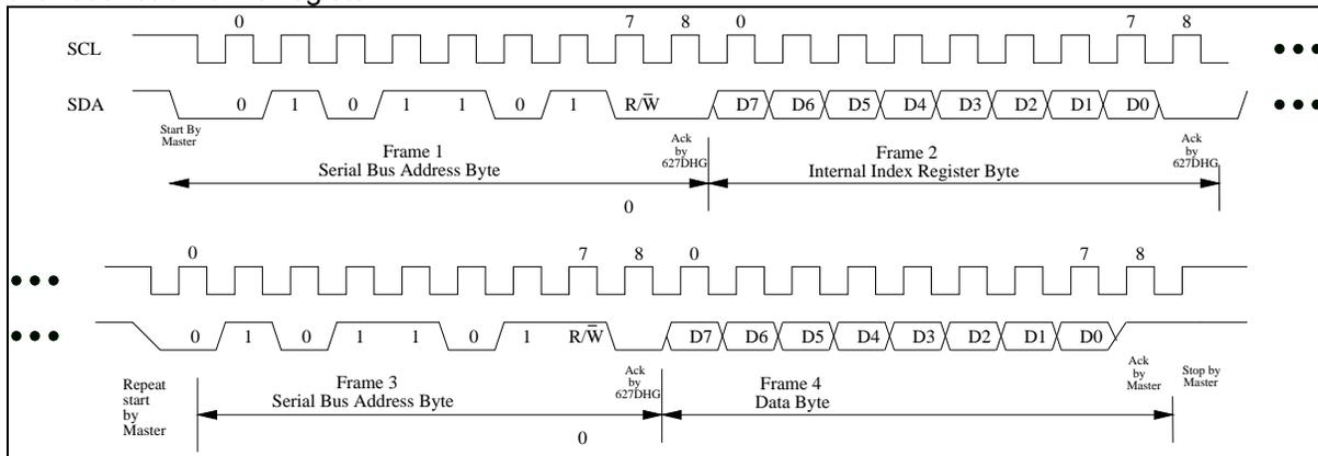
Figure 8-3 Serial Bus Read from Internal Address Register
