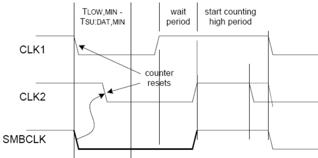
Figure 23-3 Clock synchronization
