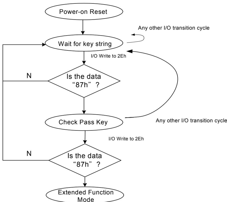
Figure 7-2 Configuration Register
