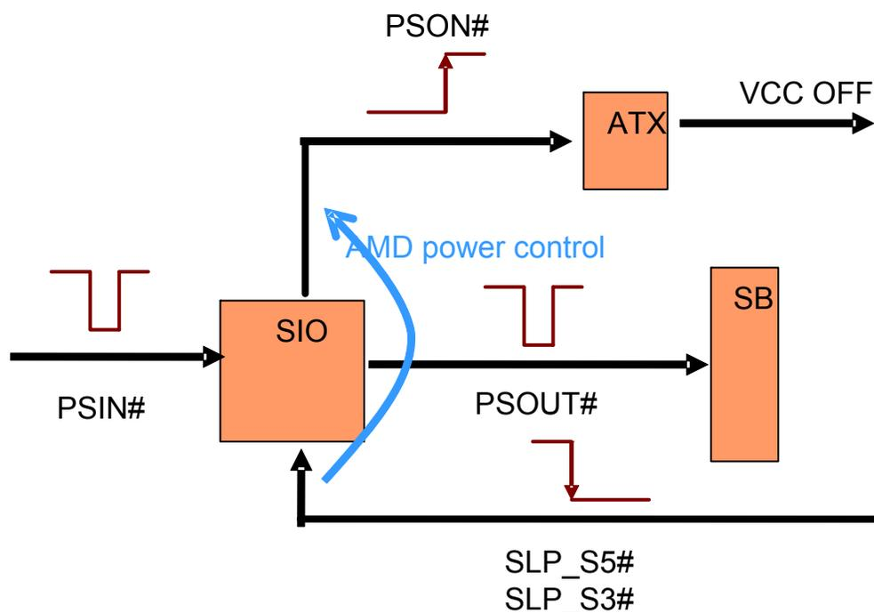
We support new AMD power on sequence base on ACPI power on sequence , therefore , user can choose which architecture by set the strapping pin GP25 . If GP25 is 0, only ACPI power on sequence is set , otherwise, AMD power on sequence is combined with ACPI, user can set CR2F[5] to get the same condition. To make sure CR2B[4]:GP34\_SEL and CR2B[0]:GP30\_SEL are "0" before running the sequence, because they are ATXPGD and SLP\_S5 pin select.
