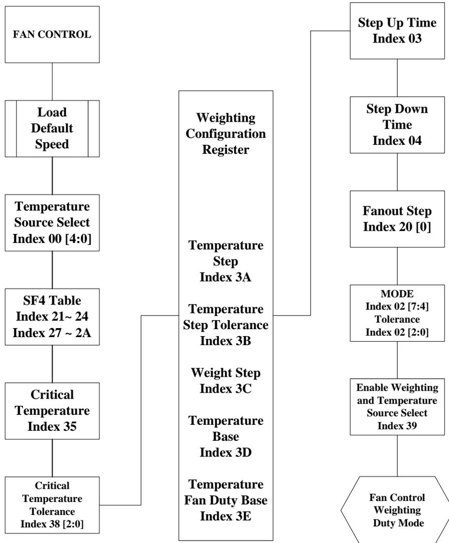
Figure 8-17 Fan Control Weighting Duty Mode Programming Flow
