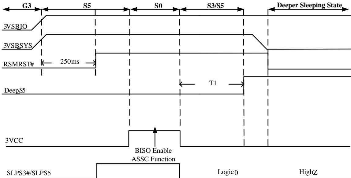
When the first time AC plug in and enter into S0 State, BIOS can enable ASSC Function (DeepS3 or DeepS5), when the system enters S3/S5 state, the pin DEEP\_S5 will be asserted after pre configuration delay time (power\_off\_dly\_time, LD16 CRE2) to make the system entering the “Deeper Sleeping State (DSS)” where system’s VSB power is cut off. When pin DEEP\_S5 asserts, the pin RSMRST# will de-assert by detecting PSOUT# signal (monitor 3VSB SYS Power).
